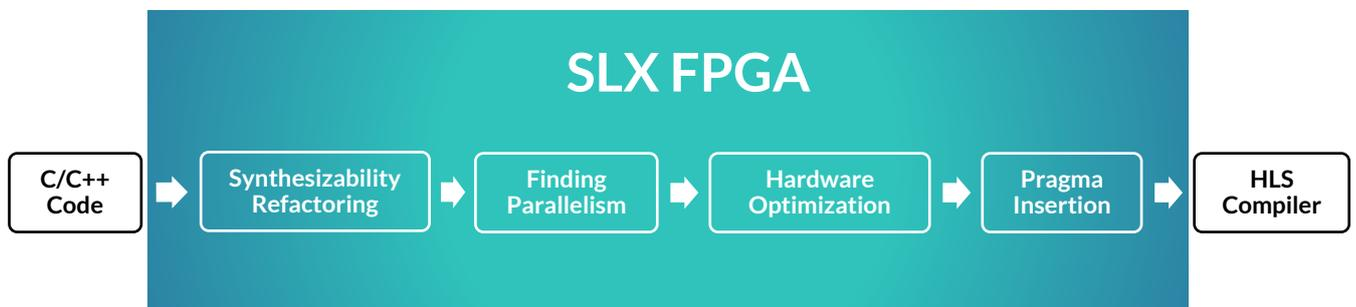
Figure 2: SLX FPGA workflow from a generic C/C++ code to a HLS ready code optimized for HW implementation.
